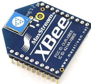
Having encountered technical issues using a star network, I decided to communicate Xbee devices through **end-device** to **end-device** communication using a broadcast emission. This issue is proper to low level OSI layers. Thus, it doesn't affect the application level, it can be fixed without worrying about the code behind it.
